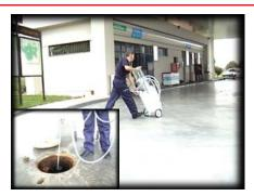
Close the air valve and place the extractordecontaminator close to the container. Take down the probe until its bottom.
