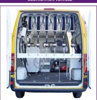
Personalized installation of kits for the lubricant transfer assembled into a van. It allows the lubricant, grease and air compressed supply through the hose-reels. The meter nozzles control the supplied amounts. It also allows the waste oil suction from a recuperator to a residual tank placed in a box of the van.
